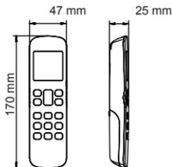
Figure 2.1 Dimensions of remote controller
